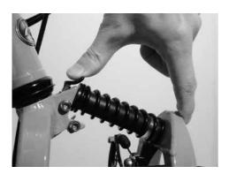
• Fold the front swingarm right under until the front wheel rests next to the main frame tube, and the tire grips up against the fixing screw on the front forks.
