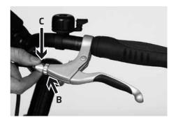
Take care that the slot of the adjustment screw is not orientated to top or front.
