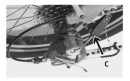
Loosen both axle nuts and remove the rear wheel.
