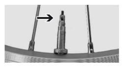
If the presta valve is not sufficiently tightened, this leads to the gradual loss of air. Check the tightness of the of the valve body in the elongated shaft. Make sure the valve diameter matches the hole in the rim and that the valve stands up straight.
