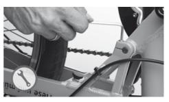
The clamp bolts must be tightened to 5 Nm torque.
