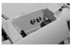
The M 6 x 12 bolt is secured into the main frame with threadlock adhesive. The bolt should be screwed in just far enough that when the catch is engaged, it's under slight tension inwards.
