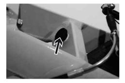
Fold the front swingarm right under until the front wheel rests next to the main frame tube, and the tire grips up against the fixing screw on the front forks.
