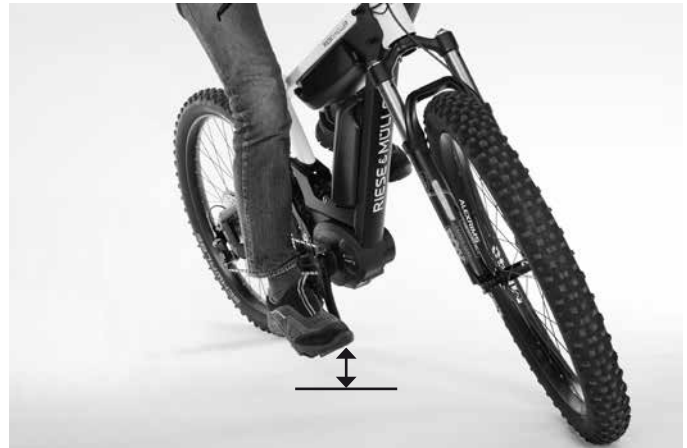
Hazardous: Crank arms not horizontal
