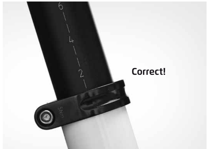
Correct: Hidden minimum insertion mark of the seat post
