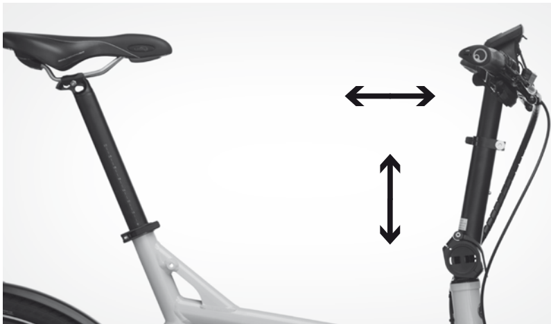
Stem with height and angle adjustment
