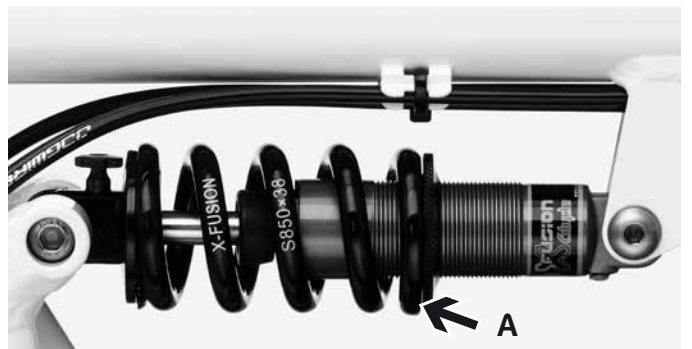
Rear shock absorber with steel spring
