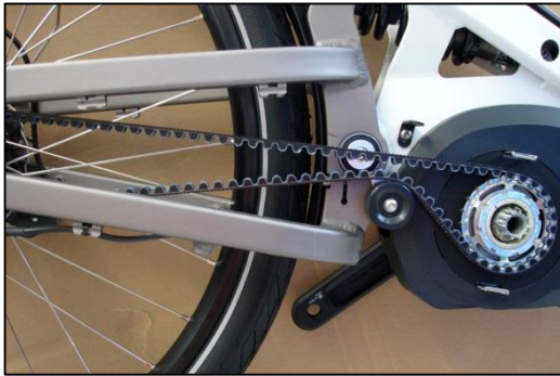
fig. 4: checking the belt tension
