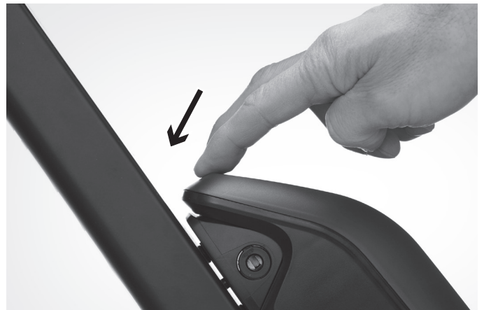
Press battery into locked position
