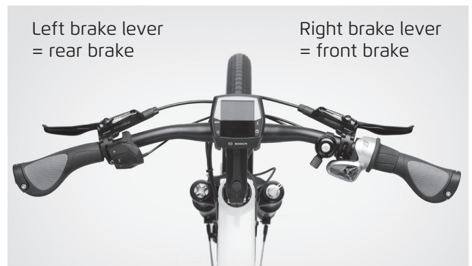
Modified set-up (brake cables switched), if so desired
