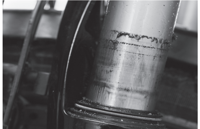
Oil leakage at the fork
