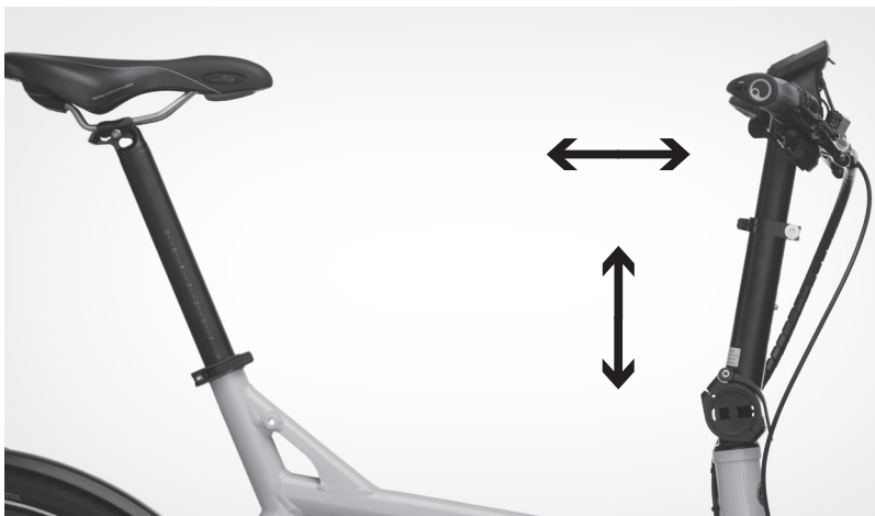
Stem with height and angle adjustment
