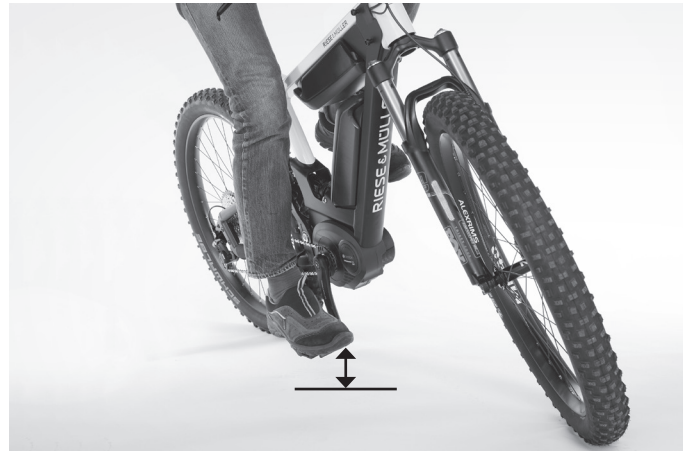
Hazardous: Crank arms not horizontal
